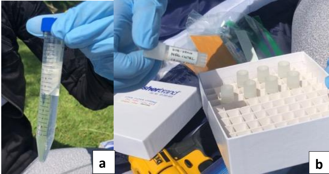
Figure 9. Storing filter in liquid preservative in either a) 15 ml falcon tube or b) 2 mL screw-top tube, both pre-filled with liquid preservative.
