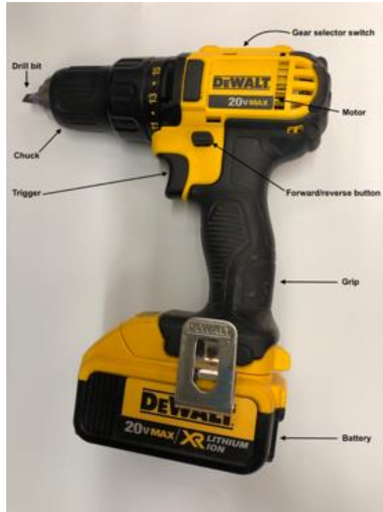
Figure 2. Components of cordless drill
