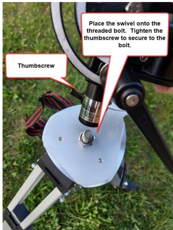
Figure 12. Attachment of tripod swivel to tripod.
