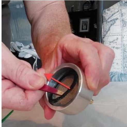
Figure 16. Removal of rubber gasket with sterile forceps.
