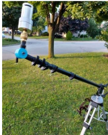
Figure 14. Position of inverted filter housing for purging stage.
