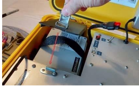
Figure 8. Fitting of battery into compartment.
