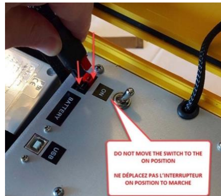
Figure 10. Plugging in battery to OSMOS unit.
