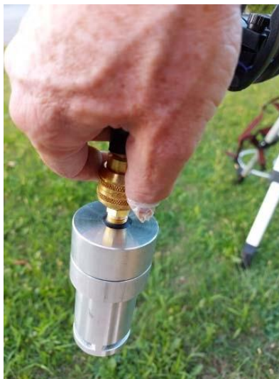
Figure 15. Disconnecting filter housing from quick connect collar.
