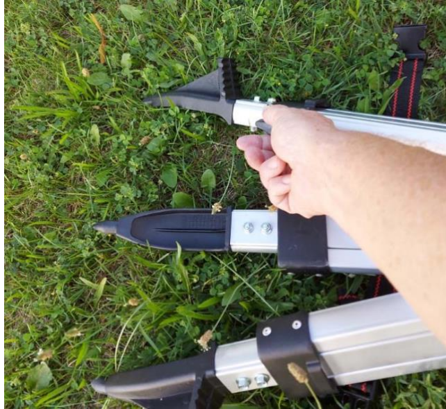
Figure 11. How to extend and adjust tripod legs.
